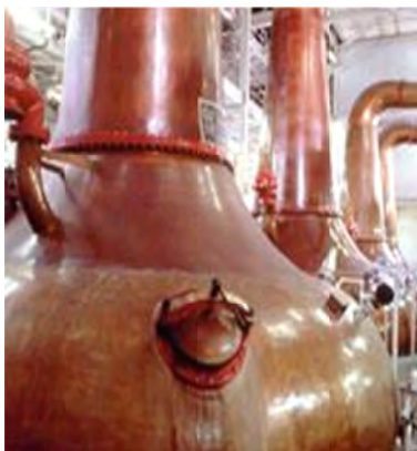
Fig. 15.1 Copper stills for batch distillation of whiskey and brandy
