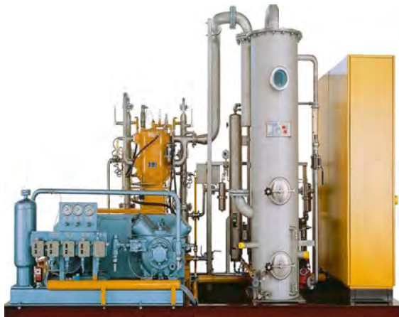
Fig. 12.43 Carbon dioxide recovery plant (brewery CO 2 )
